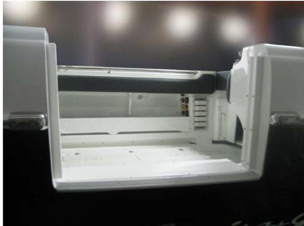
The side “dive door” is available as a portside only option. This is because the starboard side carries all of the electronics, battery and engine cabling between the helm and the transom.
