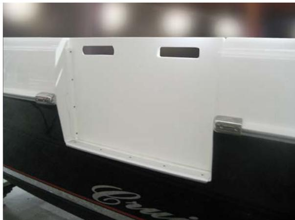
Each side “dive door” is supplied with a fully removable side door panel as well as a nylon door insert. The fibreglass moulded panel maintains the side profile and coaming profile of the hull, while the nylon insert is perfect for days at sea chasing the large pelagic fish species.
